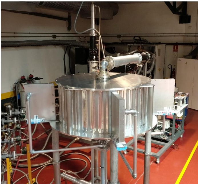
Fig. 17. Cavity combiner prototype in the CIEMAT High Power RF Laboratory
