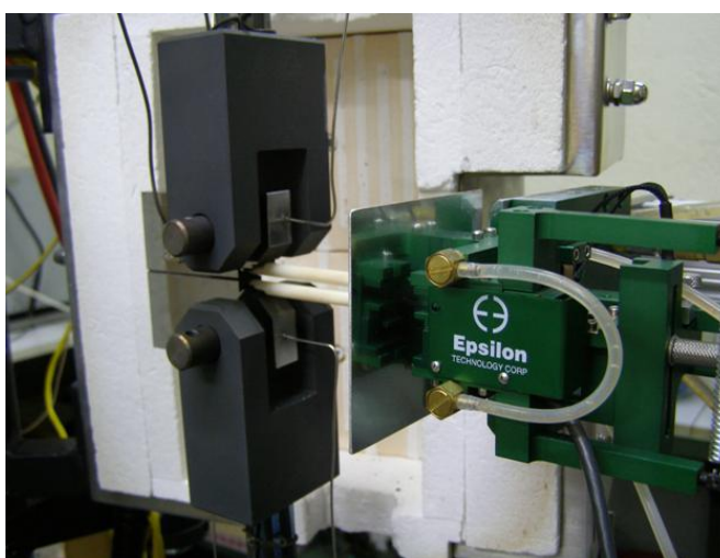
Fig. 19. Crack growth rate measurements under creep-fatigue conditions
