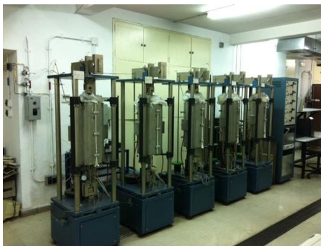
Fig. 18. Creep tests under aggressive environment
