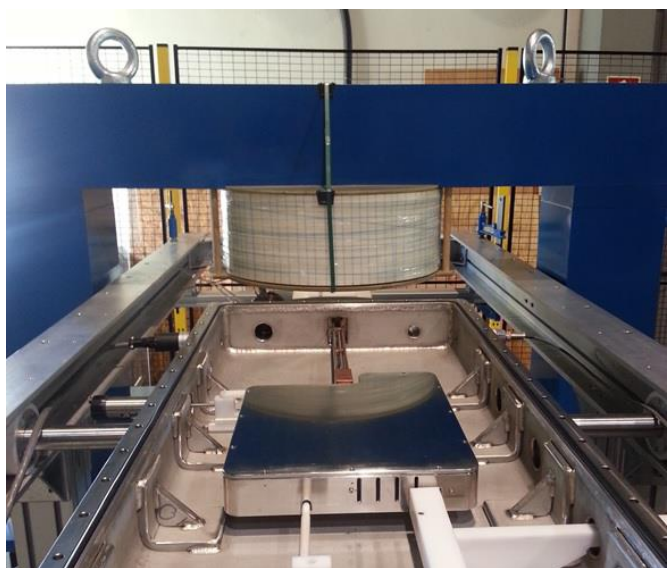
Fig. 6. A top view inside the vacuum chamber, showing the electrical shielded box, the ion source and the magnet
