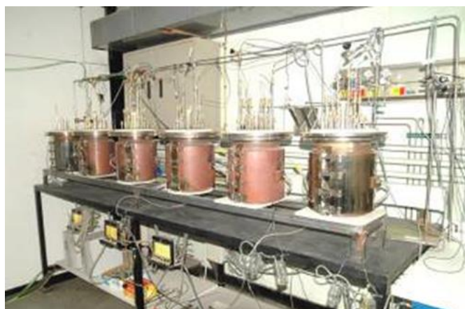
Fig. 23. Static autoclaves for high temperature immersion test in molten salts
