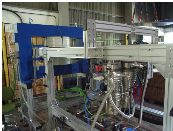
Fig. 5. Overview of the test bench with the mechanical structure, the magnet, the vacuum system, and the refrigeration water distribution system
