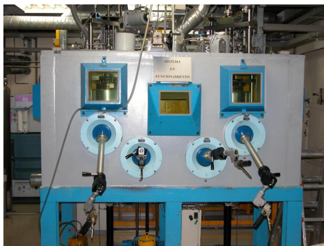
Fig. 25. HALDEN facility: SCC testing facilities in BRW reactor conditions with irradiated material
