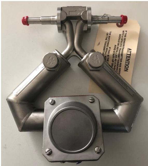
A Coriolis mass flow meter to be used in the fluid dynamics measurements
