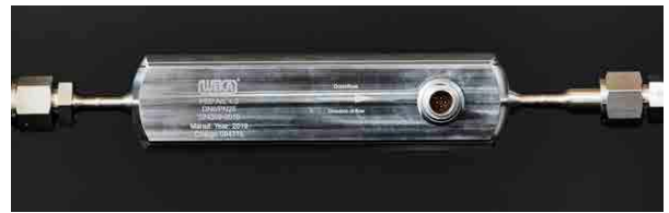
The WEKA mass flow meter to be used in the fluid dynamics measurements
