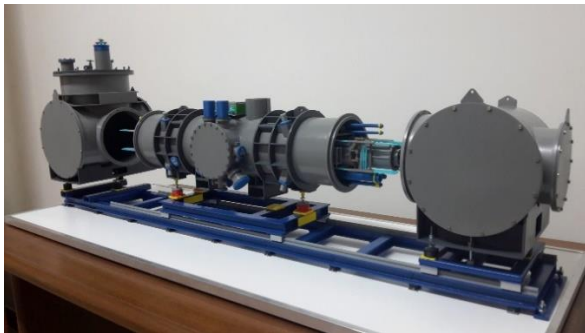
A cryogenic equipment (a quadrupole module of FAIR SIS100 synchrotron) to be tested at INFN Salerno.
